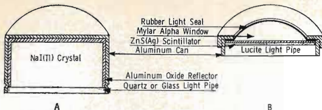
Fig. 2. Cross-sectional views of (A) gamma and (B) alpha scintillator packages showing physical and chemical makeup.
