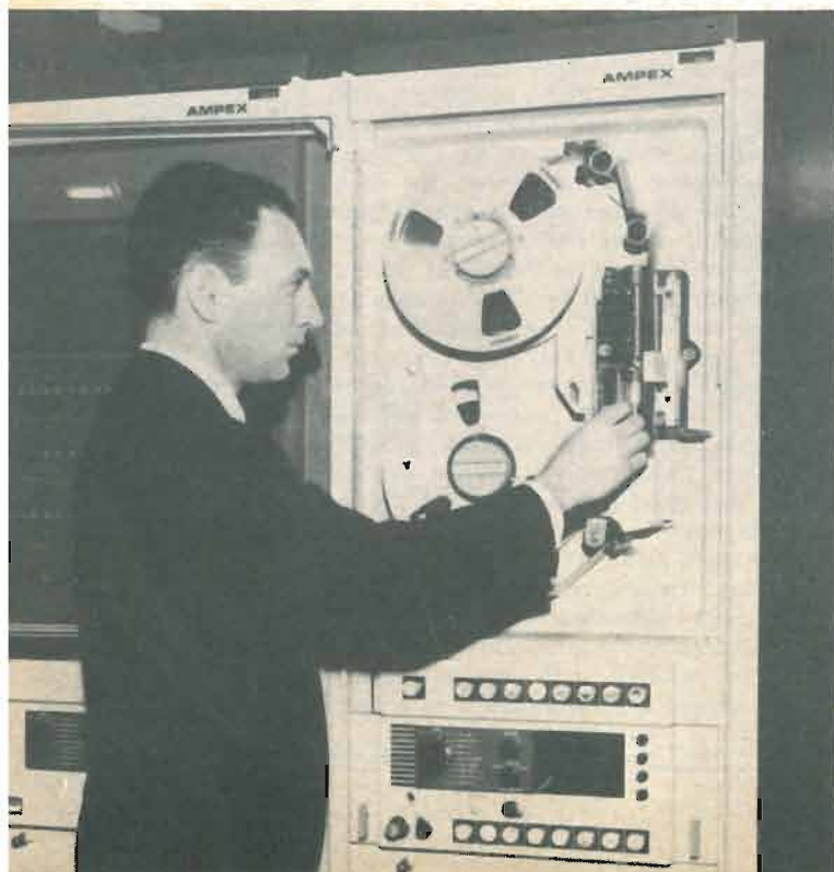
Fig. 1. FAA project engineer adjusting two-channel Ampex F-950 rotary head instrumentation tape recorder used in development of a processing subsystem for radar data to help traffic control personnel better identify aircraft during storms.
