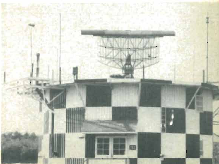
Fig. 3. FAA 60-mile range terminal radar system that will be used in conjunction with a 200-mile range enroute system to provide automated or semi-automated tracking and display of aircraft and radar weather clutter. The FAA has plans for automating such terminal radar systems at high density sites.
